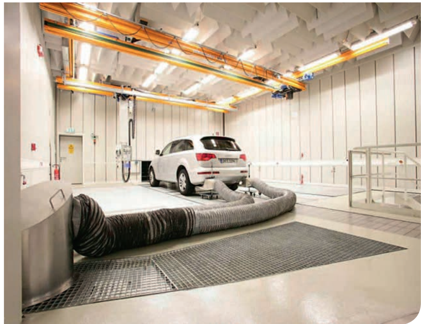
Hemi-anechoic room showing flat absorbers on the walls with wedges in the roof to increase the amount of absorption
