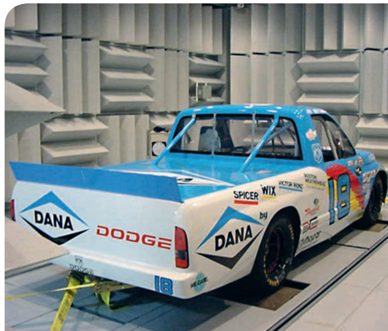
Hemi-anechoic chamber for Dana Trucks, USA
