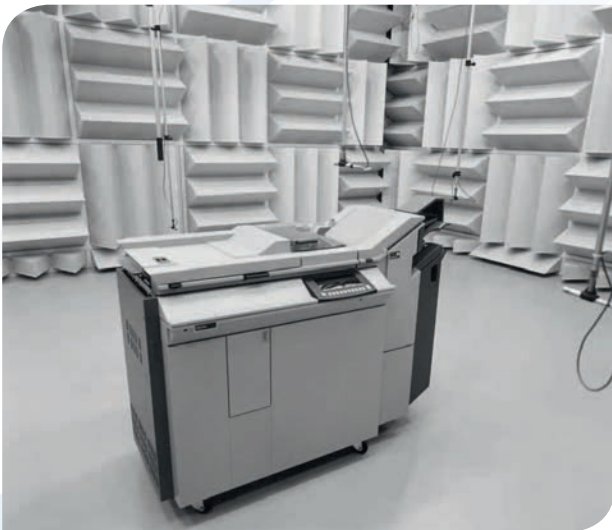
Hemi-anechoic chamber for OCE for testing printers and other office machines
