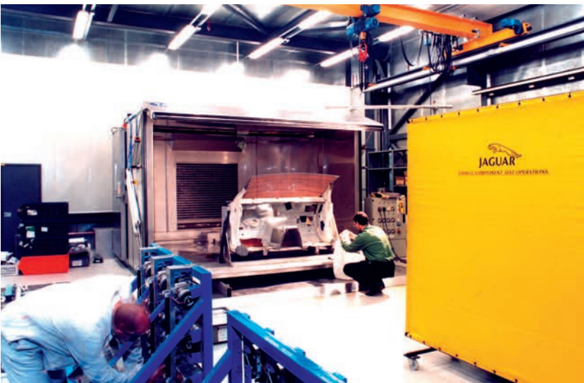
Airbag in-vehicle testing chamber, Jaguar, UK
