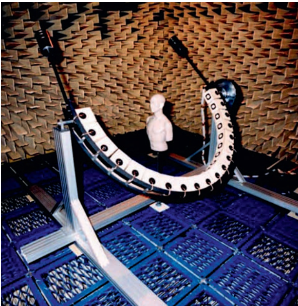
Example of Microdyne® fully anechoic chamber with grated floor for ISVR in Southampton
