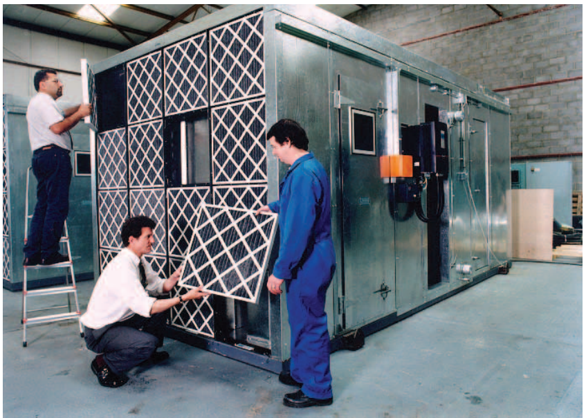
IAC acoustic AHU during assembly
