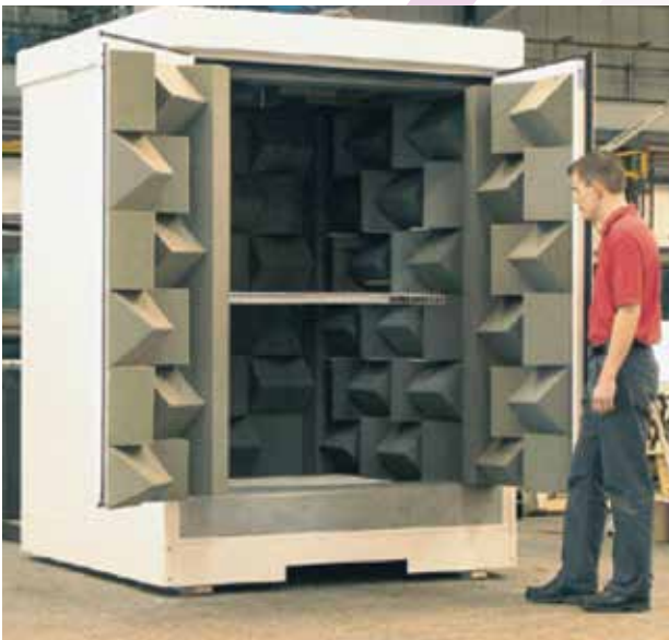
Example of Microdyne® mini anechoic chamber during use
