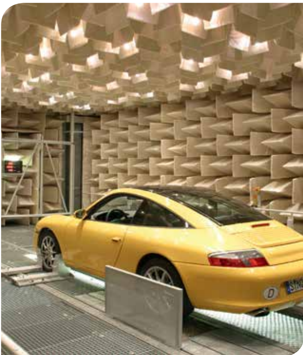
Fully anechoic chamber with 4x2 dynamometer for Porsche, Weissach, Germany
