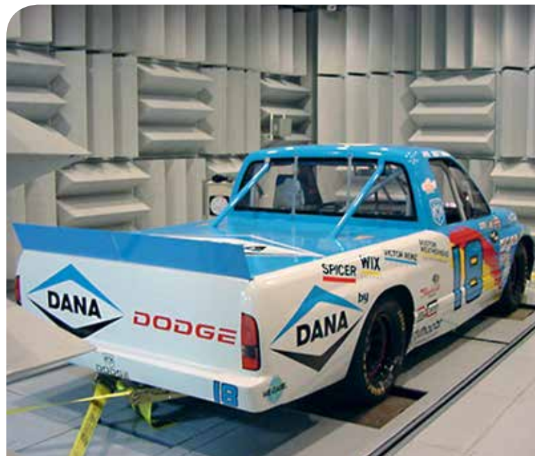
Hemi-anechoic chamber for Dana Trucks, USA
