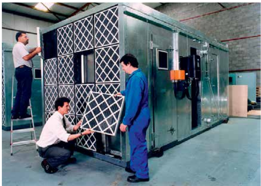
IAC acoustic AHU during assembly
