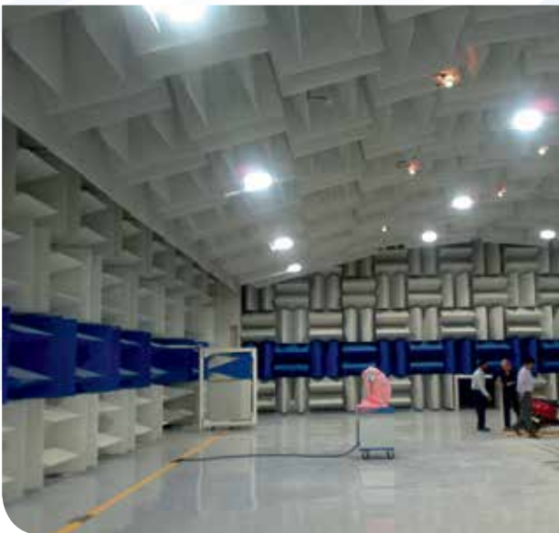
Hemi-anechoic pass-by chamber for Bajaj Motorcycles, India
