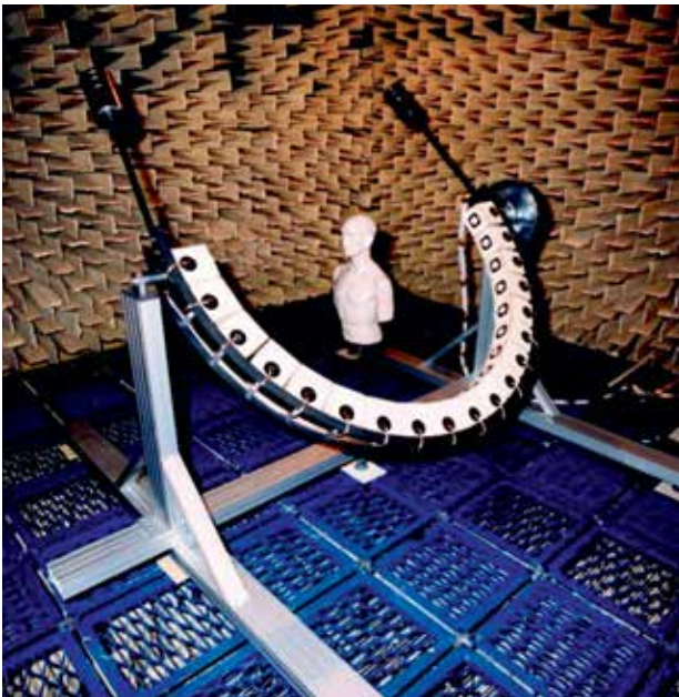
Example of Microdyne® fully anechoic chamber with gridded floor for ISVR in Southampton
