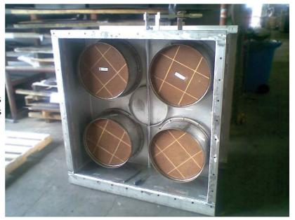
IAC Acoustics purchase substrates and fabricate the housings to suit the application. The substrates can be full soot filters or simple oxidising catalysts. They can be tuned to suit marine diesel or on road diesel.
