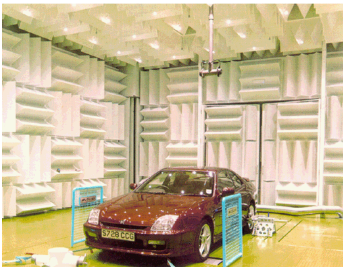
Vehicle Semi-Anechoic Chamber (VSAC), Tennex Europe, UK
